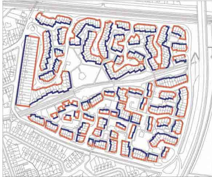
Figure 28 Fronts and backs of homes as existing (blue is 'normal' front doors, albeit often facing quiet spaces; red is 'backs' exposed to public access)
