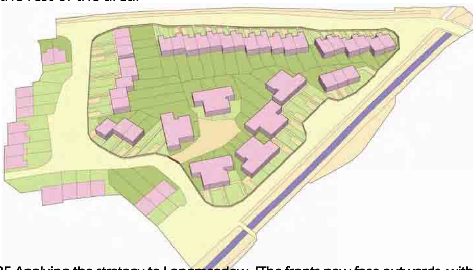
Figure 35 Applying the strategy to Longmeadow. [The fronts now face outwards, with their own front gardens. The courtyard may be retained for servicing and access to (e.g.) an 'extra care' unit in the remaining 'internal building'.]
